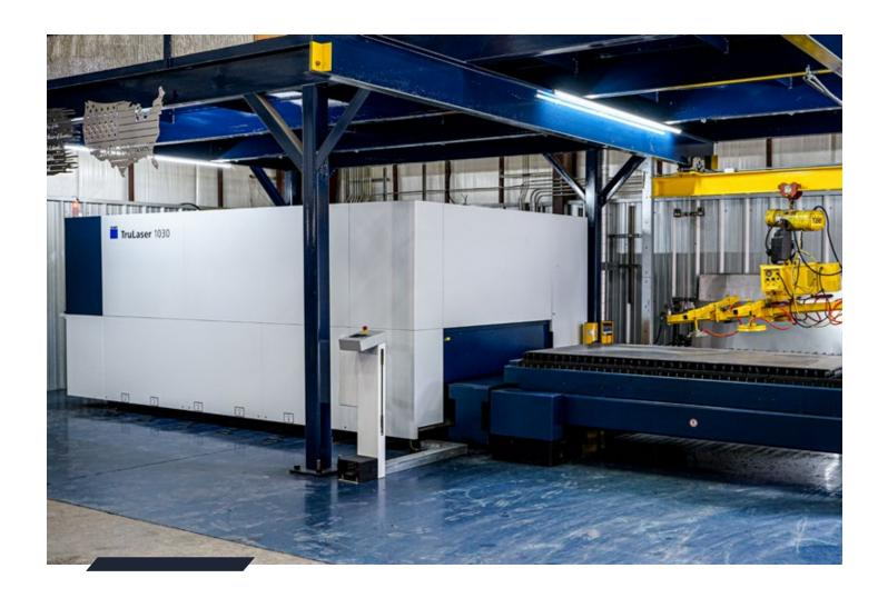
Triofab Inc. invested in a new Trumpf TruLaser 1030, giving the company 6 kW of laser power at the price of a 2-kW machine.
