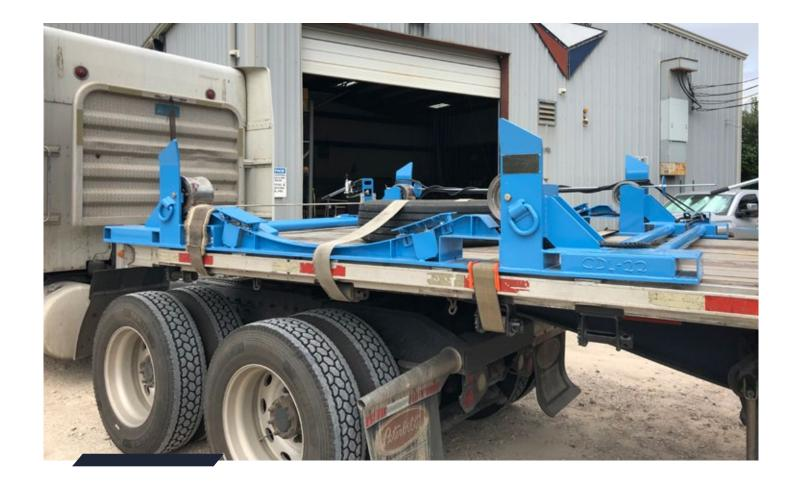
Triofab Inc. started as a specialist in custom machinery builds and has grown into a full-service engineering and fabricating firm, producing equipment such as the flexible tubing cradle shown here.
